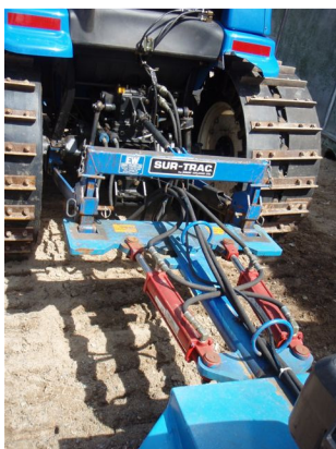
Ram steering, a close up view.
